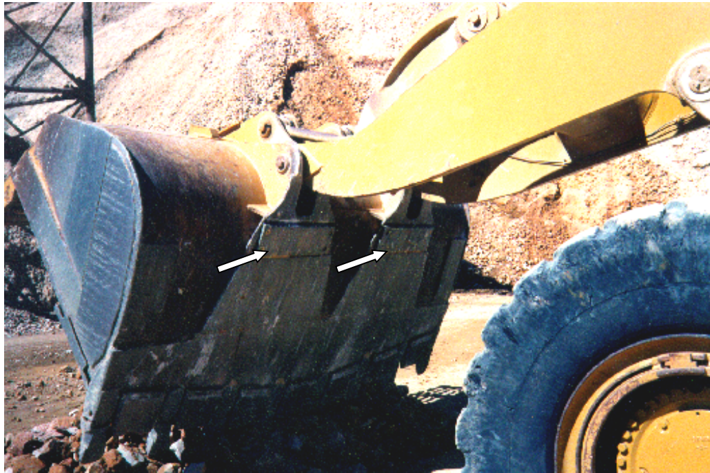
Figure 5.2: - The arrows show the location of the heel plates on the excavation bucket of the Caterpillar 988F wheel loader.
