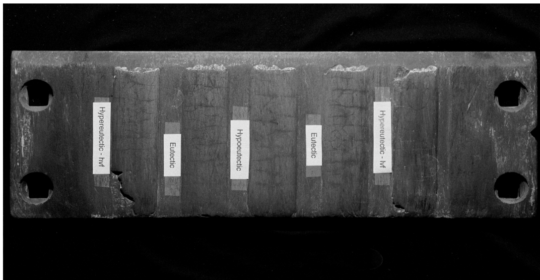
Figure 5.6: - A heel plate after service.
